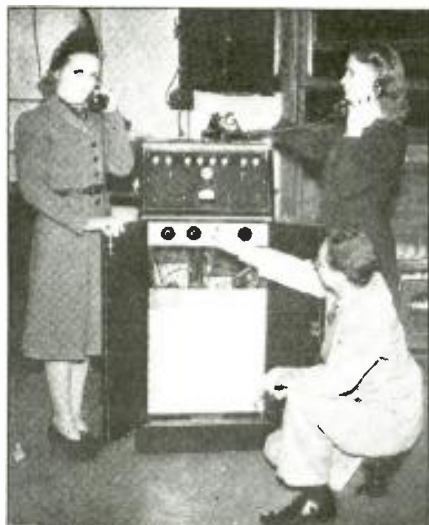
At the turn of a switch, this gadget simulates a telephone dial tone, busy signal, 20-cycle ringing, etc. You may have heard this device operating in the new air program, "The Shadow", over the WOR Mutual network.
